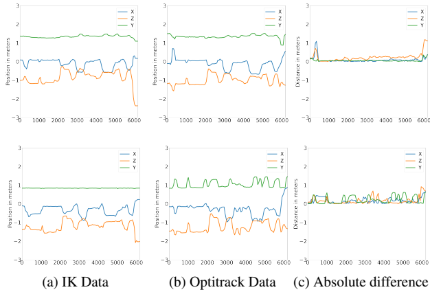
Figure 8: Transform data of the right (top row) and left (bottom row) wrists transformations from a single user during the pointing task, while observing their Optitrack avatar, and the absolute difference between the IK and Optitrack avatar transforms.
